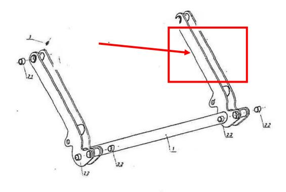
Stamped on flat surface on Lift Arm on Power Pack side
