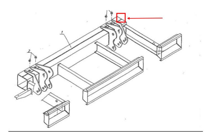
Stamped on top of main frame assembly (flat part) at mounting brackets on Power Pack side
