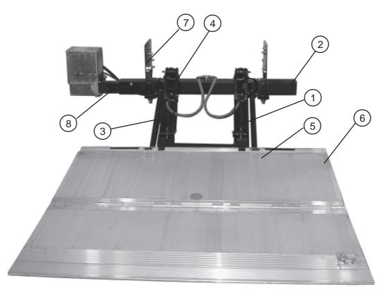
The main frame (2) is mounted to the vehicle chassis with the mounting brackets (7).
