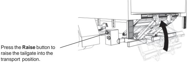
**ATTENTION:** AFTER REACHING THE TRANSPORT POSITION, IMMEDIATELY RELEASE THE RAISE BUTTON TO PROTECT THE TRUCK BODY.
