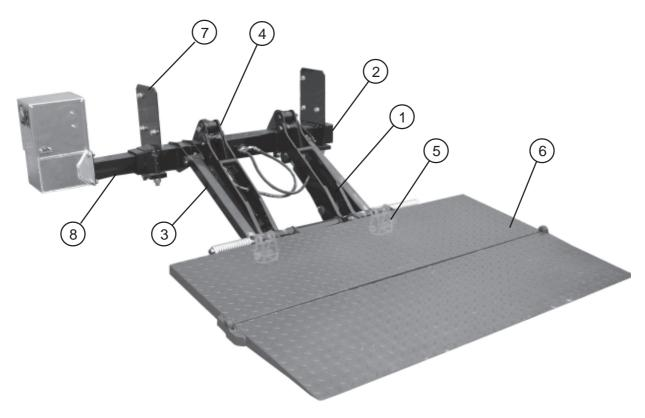
The main frame (2) is mounted to the vehicle chassis with the mounting brackets (7).
