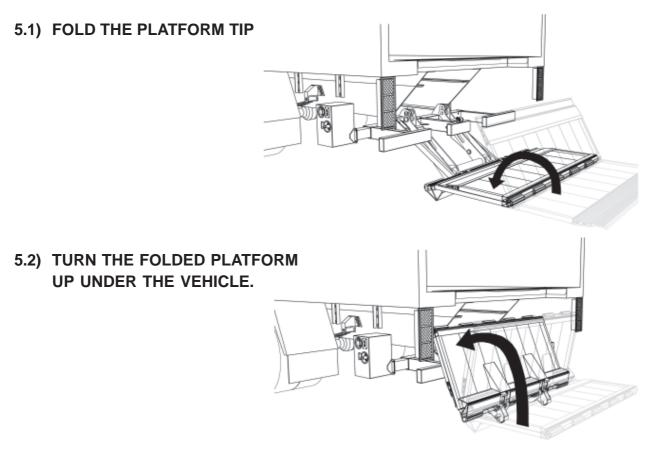
If the platform is folded (2 times), you can raise the platform to transport position.
